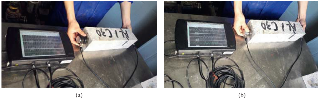
FIGURE 2: Photograph of ultrasonic velocity tests. (a) Ultrasonic compressive pulse velocity test; (b) ultrasonic shear pulse velocity test.
