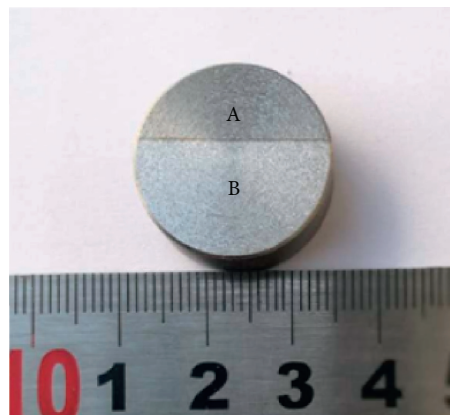
FIGURE 5: Comparison of the appearance of S0. Region A is the surface before cleaning, and region B is the surface after cleaning (200 (W)).
