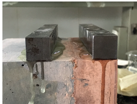
FIGURE 2: Smooth interface sample glued with two steel bar.
