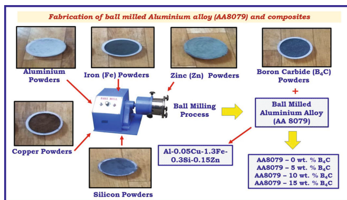
FIGURE 3: Fabrication of ball milled aluminium alloy and its composites.
