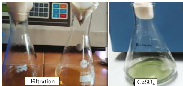
FIGURE 1: Synthesis of copper oxide nanoparticles using plant extract.
