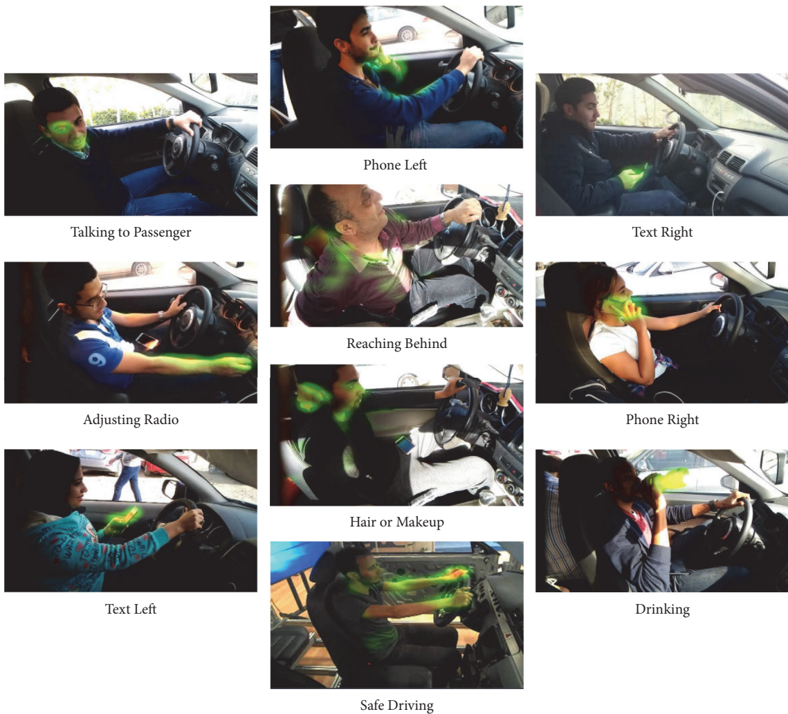
FIGURE 7: Saliency map demonstrates that our network makes its decision based on relevant features/regions in the input camera images.
