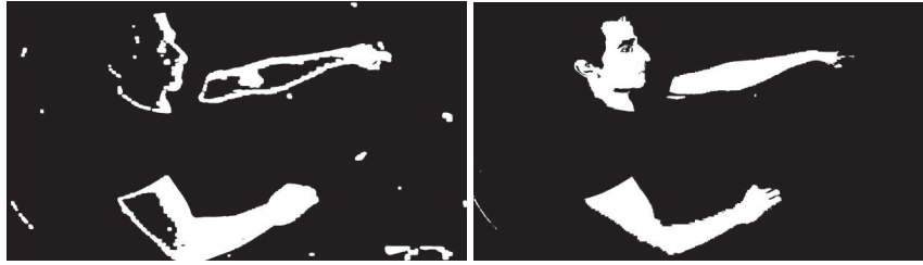
FIGURE 3: Left and right images show a sample for skin segmentation result without and with training the pixels spatial information, respectively.
