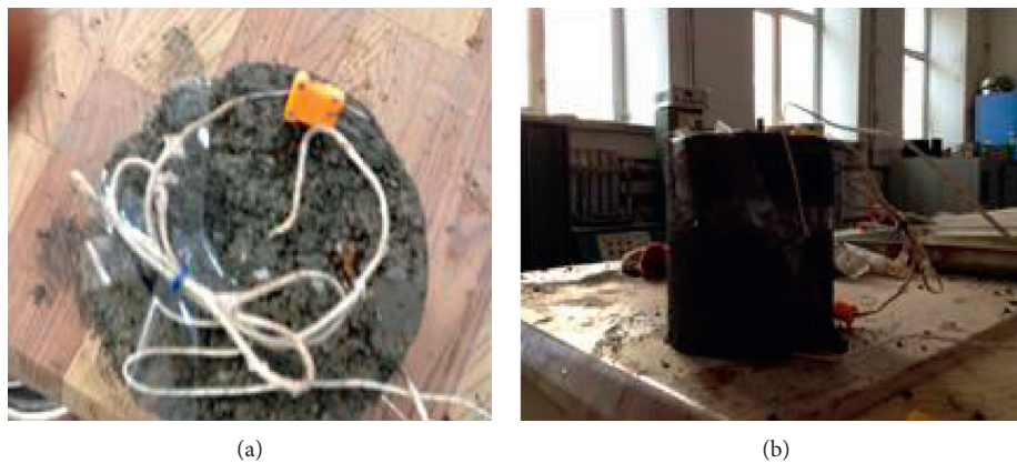
FIGURE 6: Sensors embedded in specimen. (a) Central sensors. (b) Middle external sensor.
