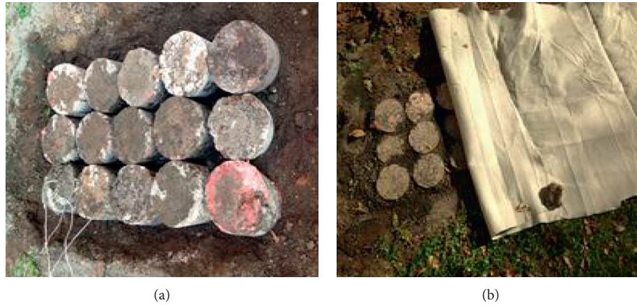
FIGURE 4: Specimen placement pictures. (a) Specimens were placed into pit. (b) Gap was filled and covered with geotextile.
