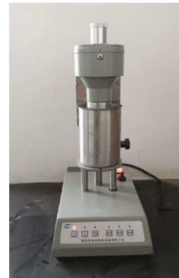
FIGURE 11: The slurry viscosity test.
