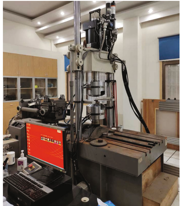
FIGURE 2: MTS-322 used for quasistatic tests.
