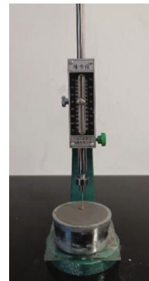
FIGURE 10: The setting time test.
