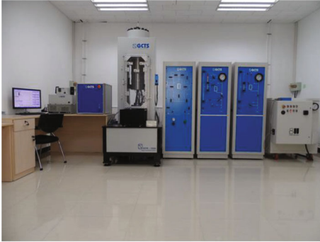
FIGURE 7: RTR-1500 Rock triaxial experiment system.
