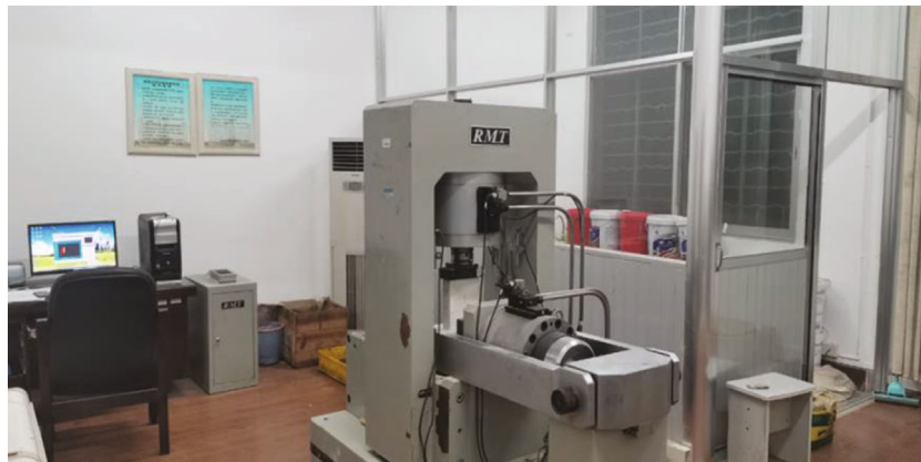
FIGURE 3: RMT-150 rock mechanics test system.
