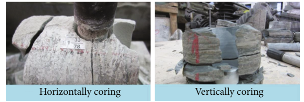
FIGURE 8: Original weak plane bedding for the drilling core.
