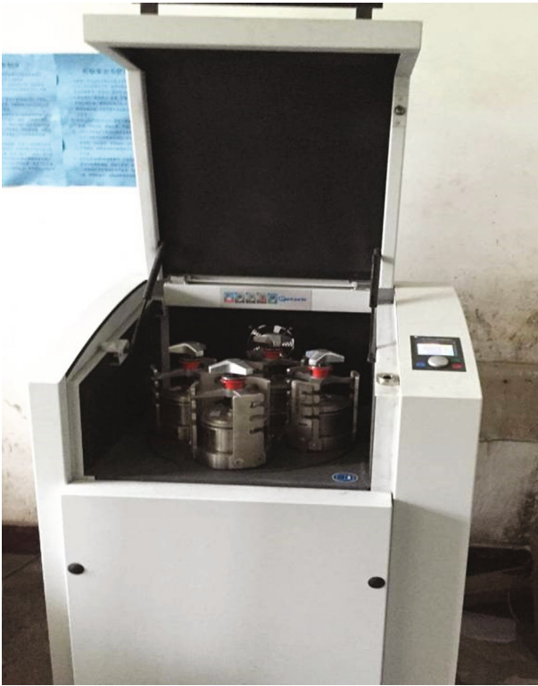
FIGURE 3: Planetary ball mill with four platforms.
