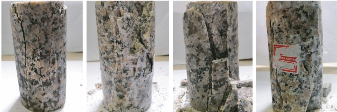
FIGURE 2: Failure patterns of granite samples after uniaxial compression tests.
