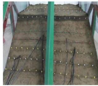
(b) Reinforced embankment model
