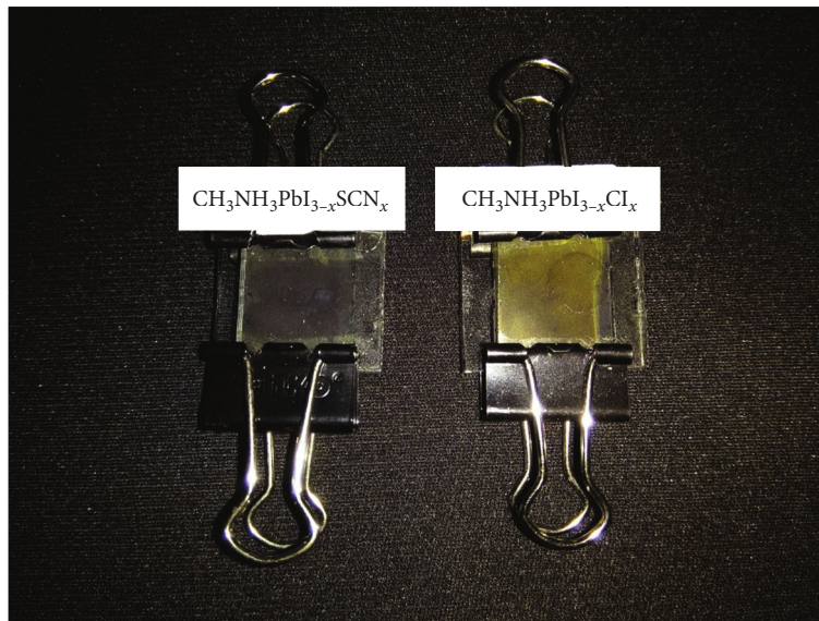
FIGURE 7: Decomposition of perovskite layer seen on day 13.
