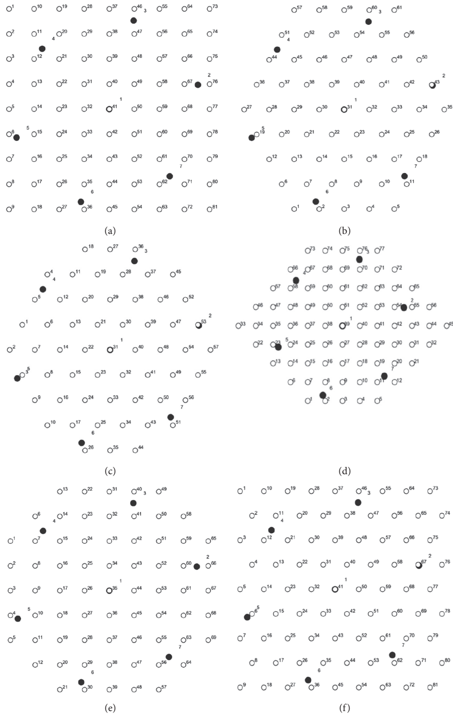
FIGURE 15: Six planar arrays; black dots are the 7-element NSA (see the text for more details).
