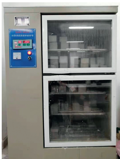
FIGURE 3: Curing of the specimens.
