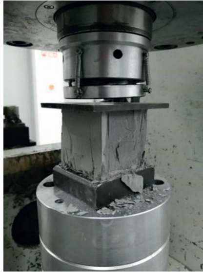
FIGURE 4: Compressive strength test.
