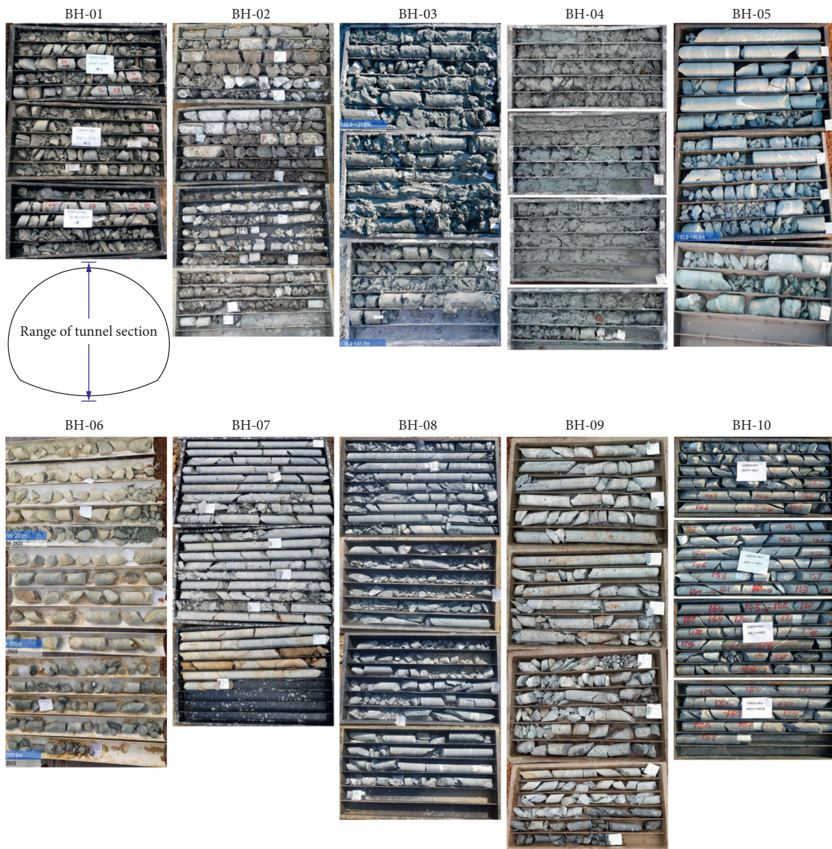
FIGURE 2: Pictures for the revealed rock mass by boreholes.
