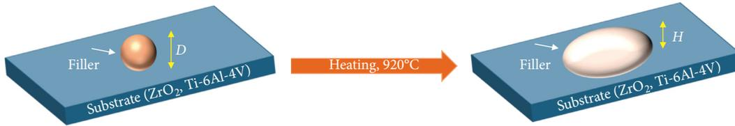
FIGURE 1: Schematic diagram for the measurement of brazeability.
