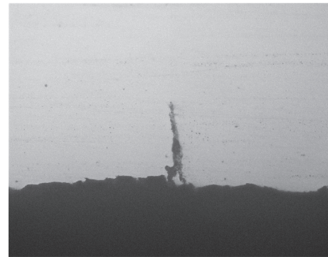
FIGURE 11: Magnified micromorphology of small distributed cracks in fracture origin area.
