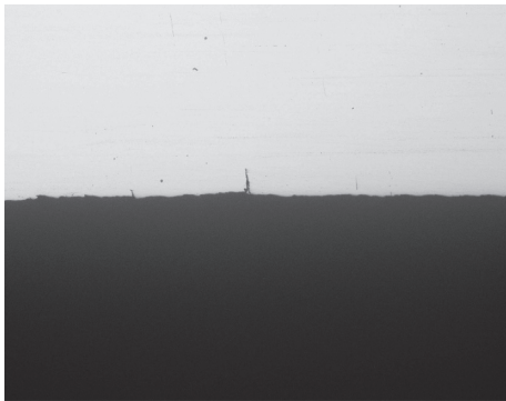
FIGURE 10: Micromorphology of small cracks.
