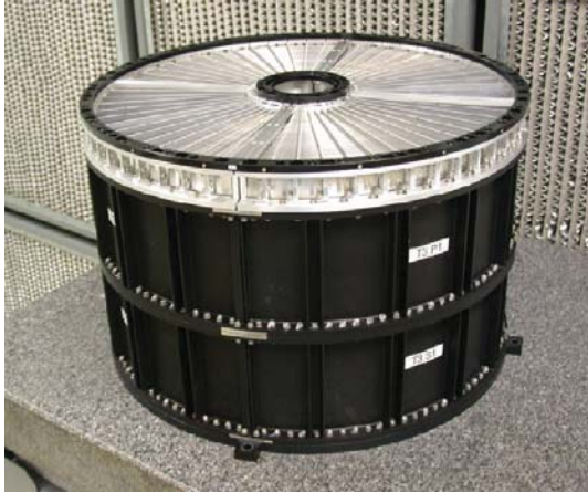
FIGURE 8: An Astro-E2 flight mirror, with stray light baffle attached on top. The aperture diameter is 40 cm; the height is approximately 22 cm. The mirror consists of 168 nested shells and has a mass of 20 kg. Between Astro-E and Astro-E2 (Suzaku) a total of 10 such mirrors were constructed.
