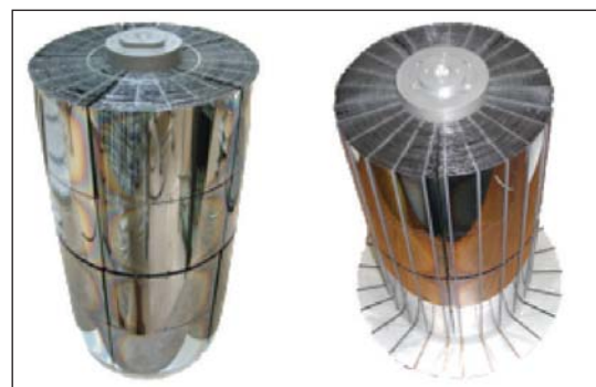
FIGURE 12: Two HEFT mirrors. Each mirror is 24 cm in diameter and 40 cm long and consists of 70 nested formed glass shells.
