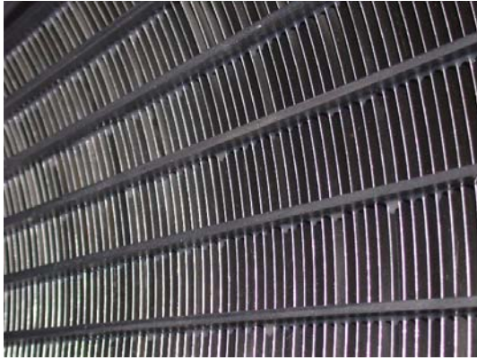
FIGURE 1: Close-up view of entrance aperture of a foil mirror. The large number of nested shells plus the use of thin foil substrates combine to provide a large filling factor. The average distance between foils is approximately 1 mm.
