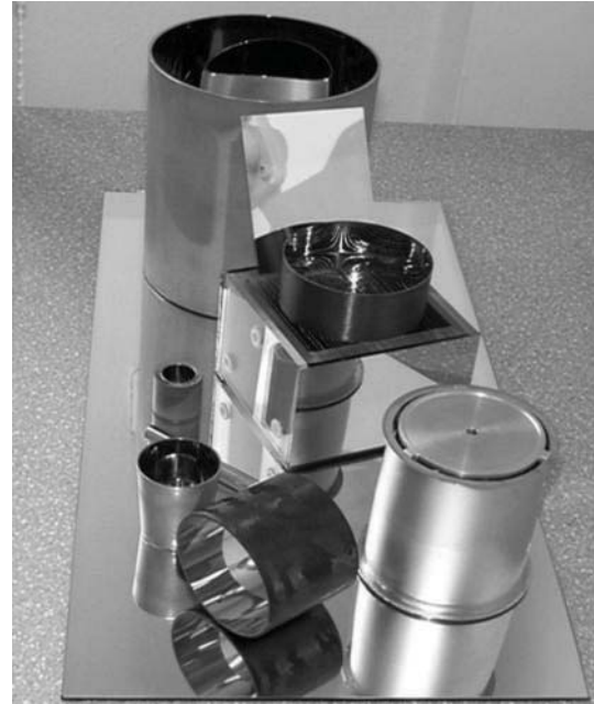
FIGURE 2: Replicated grazing incidence X-ray optics (various technologies) designed and developed by our group in the Czech Republic. The replication technology has been modified several times to meet the dedicated requirements. The two black mirrors are produced by carbon fibre technology.
