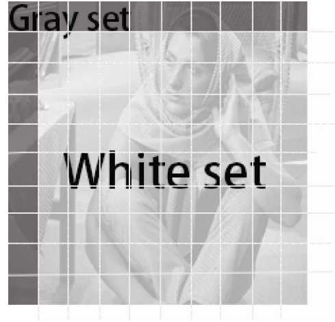
FIGURE 2: Example of image decomposing. For example, an image is sized 100 \times 100 pixels and is divided into 10 \times 10 sized block; blocks colored in gray are saved for special use, and blocks colored in white are used to embed data.
