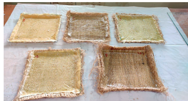
FIGURE 2: Fabrication of K/N fiber hybrid polymer composite.
