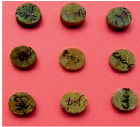
FIGURE 2: Photographic image of abrasion test specimen.
