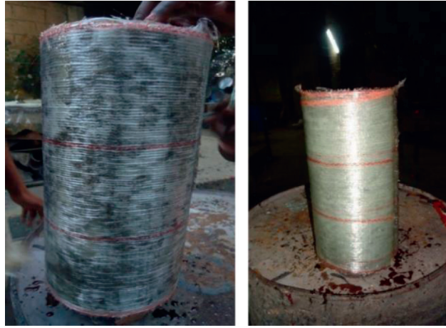
FIGURE 9: GFRP-wrapped columns.
