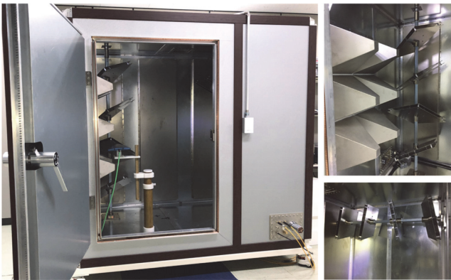
FIGURE 11: Photographs of the fabricated reverberation chamber.
