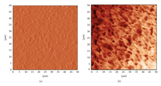
FIGURE 2: AFM images of the QCM chip. (a) Blank,  $50 \times 50 \mu m$ , (b) CNTs,  $50 \times 50 \mu m$ . AFM measurements could also be used for measuring the surface roughness of the QCM chip. The mean surface roughness was 1.0 and 2.3 nm for blank and CNTs surfaces, respectively.
