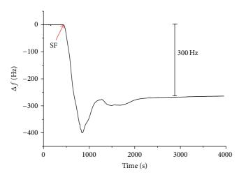
FIGURE 1: A representative of the frequency shift for preparing the electrodes decorated with CNTs/SF layer. The frequency shift of CNTs/SF exhibited the least frequency response around  $-335 \pm 21 \, \text{Hz}$ , n = 7.
