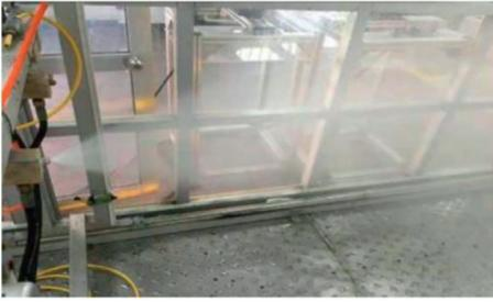
FIGURE 5: Atomization effect of 4 MPa pressure nozzle.
