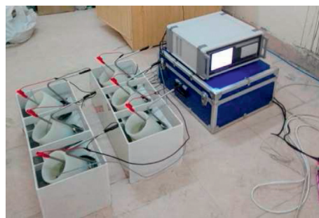
FIGURE 4: Overview of RCP testing.
