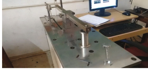
FIGURE 1: Pin-on-disc set-up used for dry sliding test.
