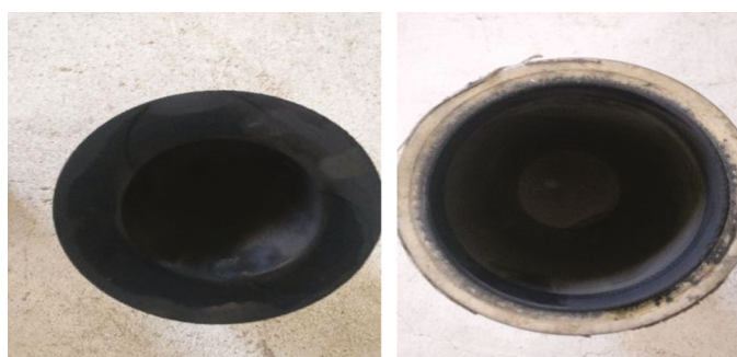
FIGURE 4: After 100 hours of operation, the piston and cylinder liner are coated.
