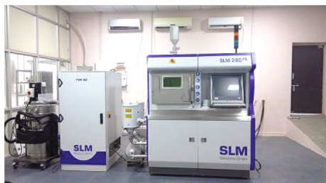
FIGURE 1: The SLM experimental setup.
