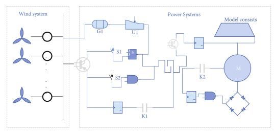
FIGURE 4: Simplified model of the power system of a wind farm.
