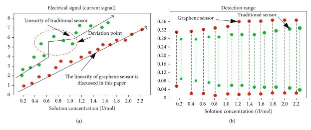
FIGURE 6: (a) Detection linearity curve; (b) monitoring range curve.
