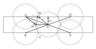
FIGURE 3: Node coverage effect diagram.
