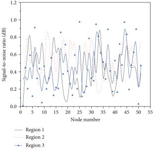
FIGURE 4: Nodal signal-to-noise ratio.
