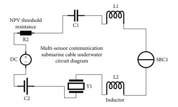
FIGURE 1: Circuit diagram of multisensor communication submarine cable underwater.
