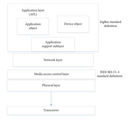
FIGURE 5: Structure diagram of a ZigBee protocol stack.
