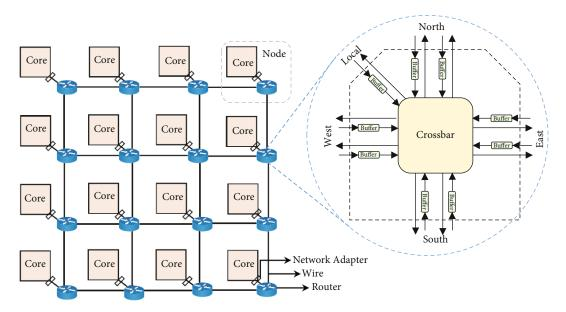
FIGURE 1: The standard  $4 \times 4$  mesh network.
