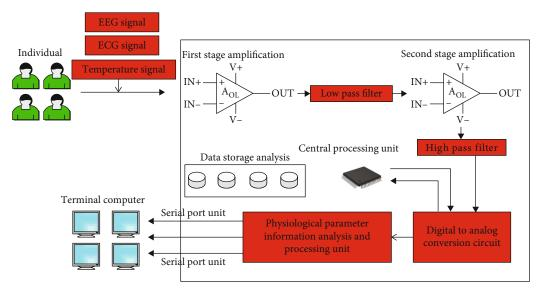
FIGURE 5: Hardware circuit principle block diagram of the data acquisition and analysis module.
