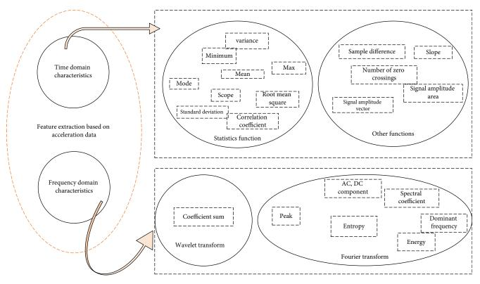
FIGURE 2: Schematic diagram of feature extraction of acceleration data.
