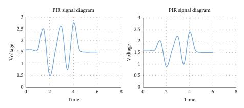
FIGURE 10: PIR signal diagram at different speeds.
