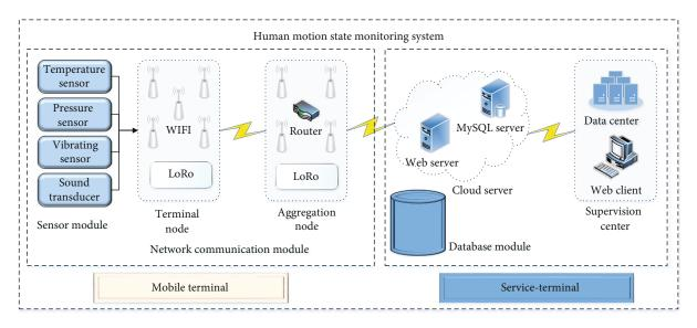
FIGURE 1: Monitoring system hardware design block diagram.
