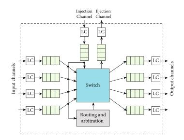
FIGURE 2: The internal structure of a router [8].
