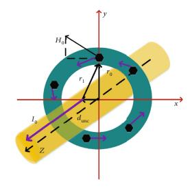
FIGURE 7: Influence of eccentricity error on annular TMR array.
