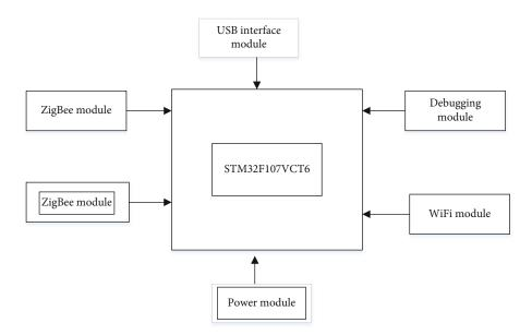
FIGURE 8: Gateway design block diagram.
