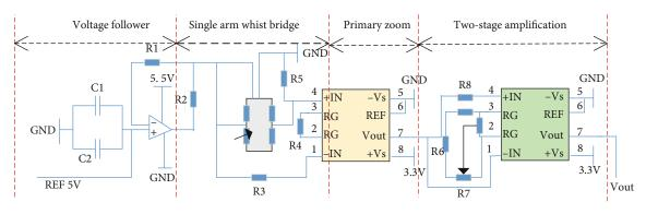
FIGURE 3: Two-stage amplifying circuit composed of AD8236.
