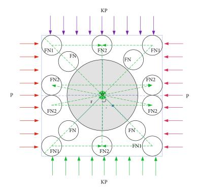
FIGURE 6: Simplified diagram of the stress distribution in the plane of the chamber under stress conditions.
