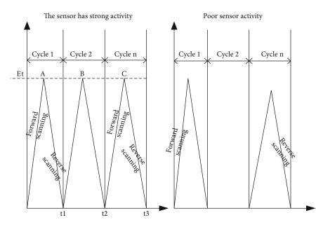
FIGURE 3: Scanning function curve of cyclic voltammetry.
