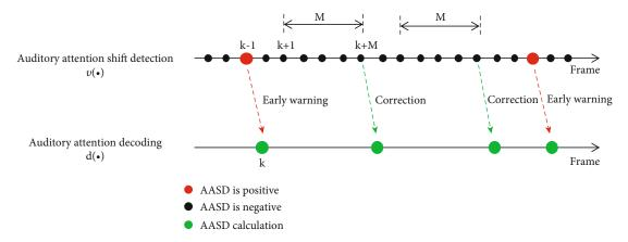
FIGURE 9: Schematic diagram of the fusion strategy of auditory attention decoding and conversion detection methods.
