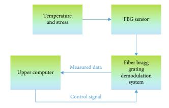
FIGURE 1: Schematic diagram of sensing system.
