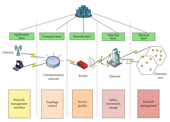
FIGURE 1: Network structure diagram of wireless sensor.
