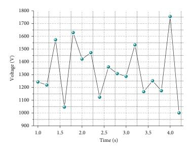
FIGURE 8: DC-side voltage for Crowbar+variable damper method.
