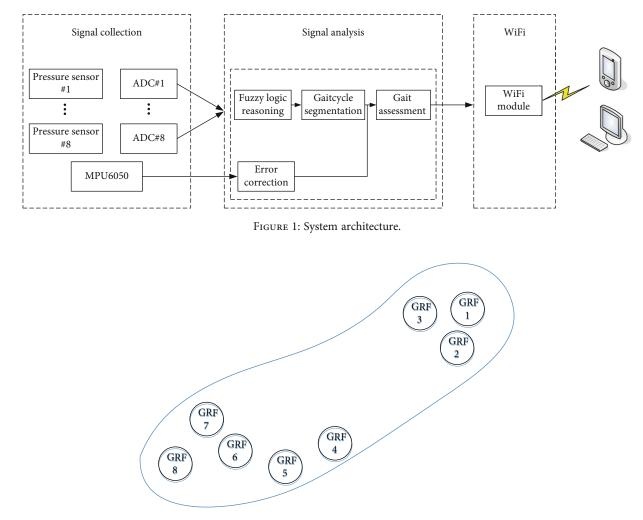
FIGURE 2: Pressure sensor distribution.
