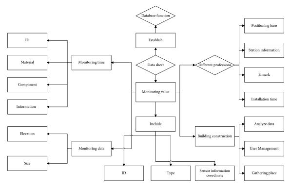
FIGURE 3: Monitoring information database ER diagram.
