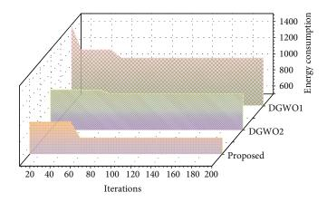
FIGURE 7: The influence of iteration times on total energy consumption of the system.
