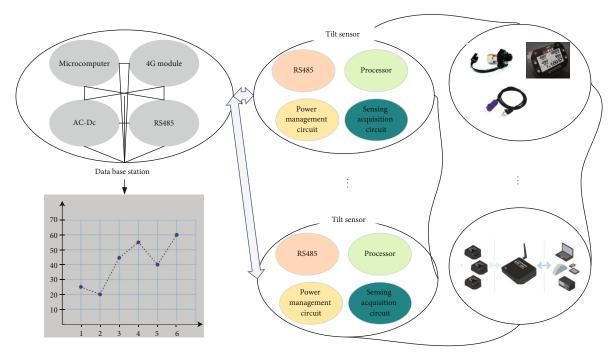
FIGURE 4: Sensor acquisition system topology diagram.
