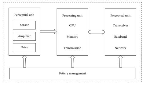
FIGURE 1: Wireless sensor network terminal node.
