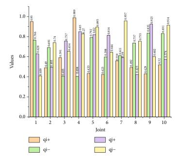
FIGURE 3: Physical limitations of the joints of the robotic arm.
