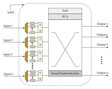
FIGURE 4: ScRN router and selection architecture.
