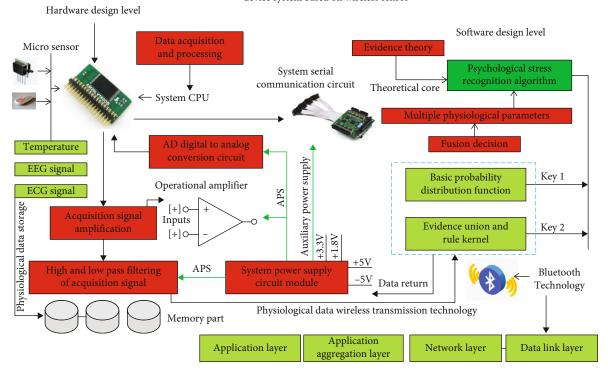
Principle block diagram of wearable psychological stress monitoring device system based on wireless sensor
