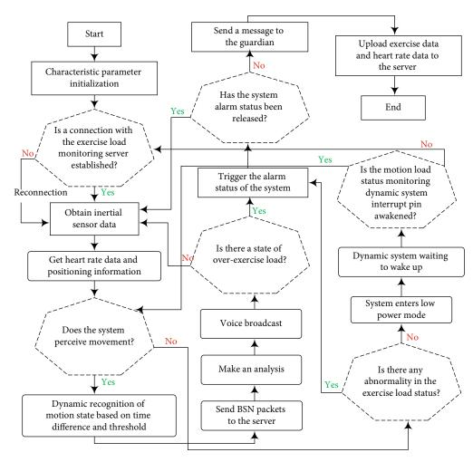
FIGURE 1: Work flow chart of the dynamic system for monitoring the exercise load state.
