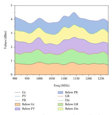
FIGURE 5: Output signal power-in, gain, and PAE test data plot.
