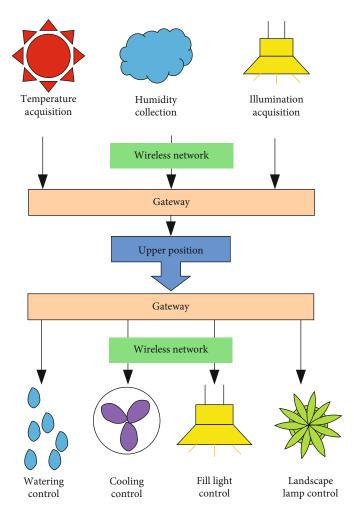
FIGURE 2: Indoor greening intelligent maintenance system structure diagram.
