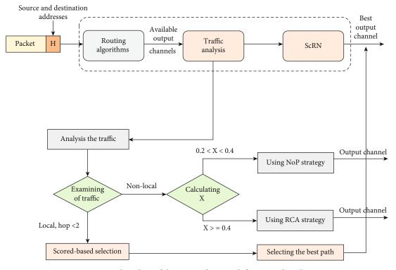
FIGURE 5: Flow chart of the proposed approach for ScRN algorithm.
