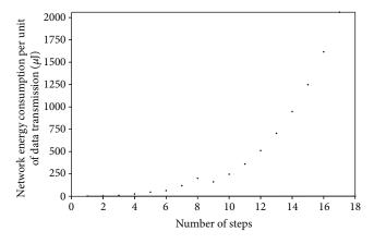
FIGURE 5: Relationship between energy consumption per unit data transmission and step length.
