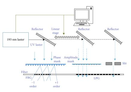
FIGURE 2: Construction diagram of fiber Bragg grating system.
