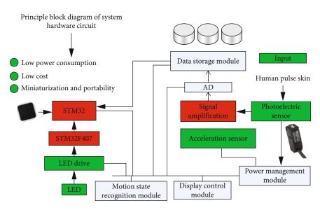
FIGURE 2: System hardware block diagram of heart rate acceleration motion wireless sensor in competitive sports.
