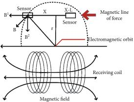
FIGURE 4: Internal setting of electromagnetic sensor.
