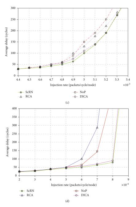
FIGURE 12: (a) Comparison of average packet latency in the transpose traffic pattern. (b) Comparison of average packet latency in the random traffic pattern. (c) Comparison of average packet latency in the hotspot-center traffic pattern. (d) Comparison of average packet latency in the hotspot-center traffic pattern.
