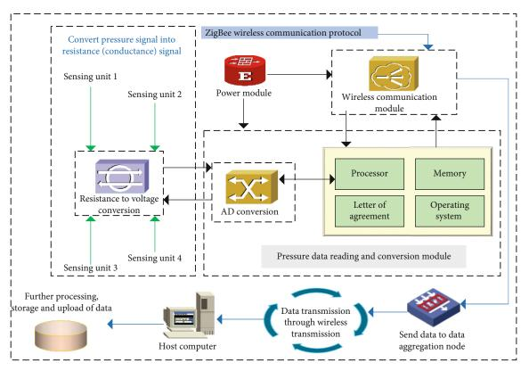
FIGURE 1: The overall architecture of flexible pressure sensor terminal hardware.
