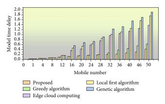
FIGURE 3: The influence of different mobile devices and different algorithms on total delay of the system.
