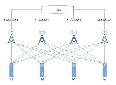
FIGURE 2: Cooperative multicell system model.
