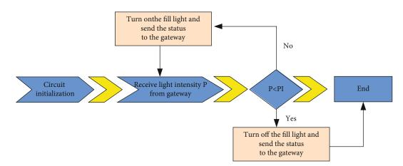
FIGURE 5: Flow chart of fill light control.
