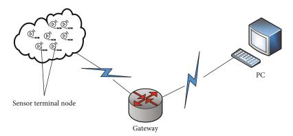
FIGURE 2: Structure diagram of a wireless sensor network.
