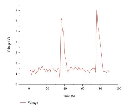
FIGURE 6: Voltage signal of energy storage capacitor.
