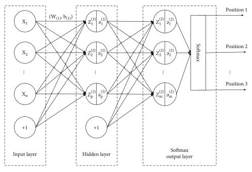
FIGURE 3: Fingerprint location model of the PIR signal position based on the BP neural network.
