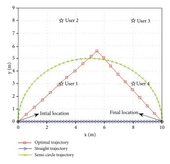
FIGURE 5: The trajectories of UAV under different schemes.
