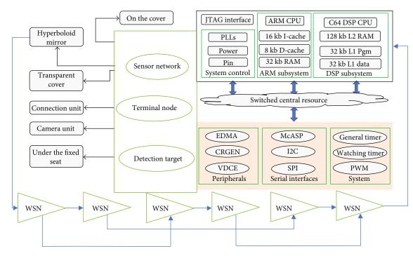
FIGURE 1: Smart sensor network topology.
