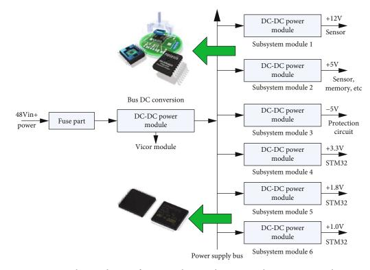
FIGURE 5: Circuit schematic diagram of power supply part in heart rate acceleration motion wireless sensor.
