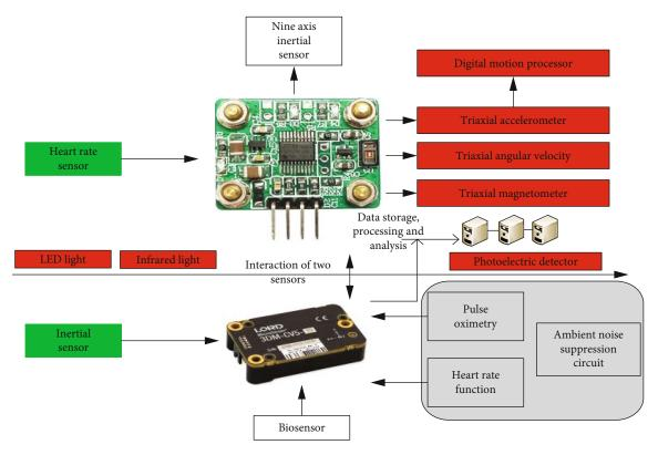
FIGURE 4: Circuit schematic diagram of sensor module in heart rate acceleration motion wireless sensor.
