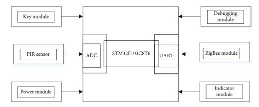
FIGURE 7: Design block diagram of an acquisition unit.
