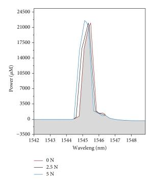
FIGURE 9: Reflection spectrum of axial force sensing.
