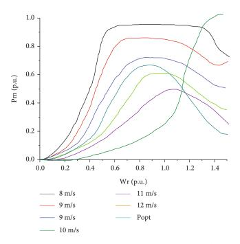
FIGURE 2: The relationship curve between the active power of wind turbine and its speed at different wind speeds.
