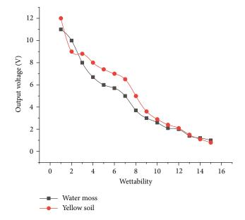
FIGURE 3: Corresponding relationship between soil humidity sensing output voltage and humidity.
