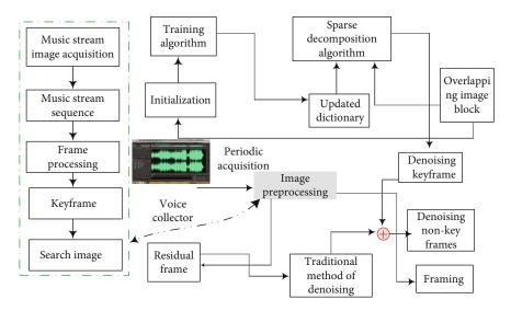
FIGURE 4: Architecture of the human voice input recognition system.
