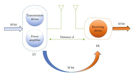
FIGURE 2: Energy consumption model.
