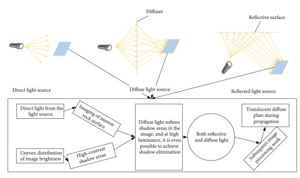
FIGURE 3: Schematic diagram of a direct light source, diffuse light source, and reflected light source.
