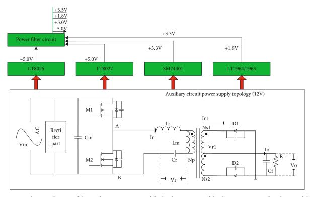
FIGURE 6: Schematic diagram of the auxiliary power circuit of the hardware system of the data acquisition and analysis module.
