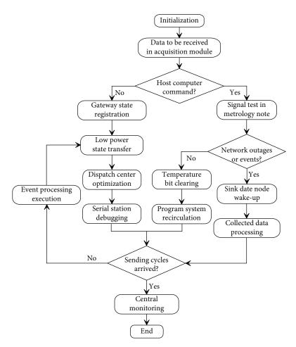
FIGURE 4: Design scheme flowchart of centralized heating monitoring system based on wireless sensor network.
