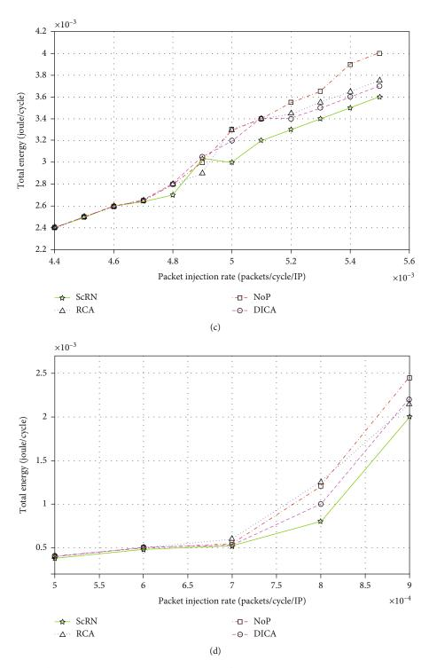
FIGURE 14: (a) Comparison of energy consumption in the transpose traffic pattern. (b) Comparison of energy consumption in the random traffic pattern. (c) Comparison of energy consumption in the hotspot-center traffic pattern. (d) Comparison of energy consumption in the hotspot-row traffic pattern.
