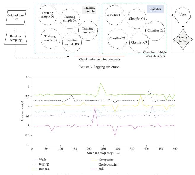
FIGURE 4: The acceleration of the sliding window segmentation when the overlay rate is 50% and the window is 100.
