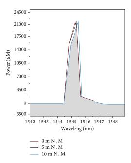
FIGURE 8: Reflection spectrum of torque force sensor.
