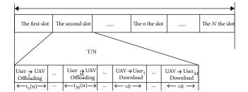
FIGURE 2: Computation offloading from user to the UAV.
