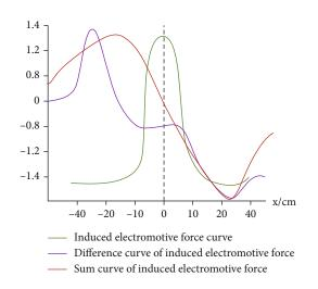
FIGURE 5: Induced electromotive force function diagram and its difference, sum value comparison diagram.
