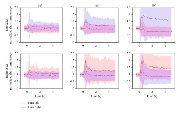
FIGURE 5: Normalized sensor NEMG short-term energy diagram (6 types of sight orientation changes).
