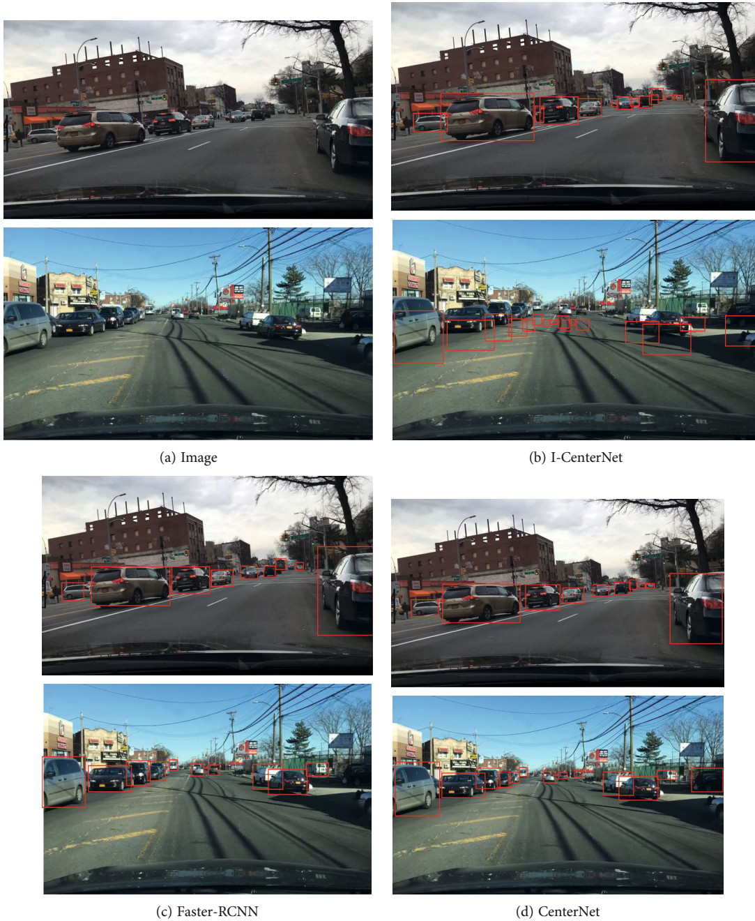
FIGURE 7: Experimental results of this article. Among them, (a) is the original input image, (b) is the improved result proposed in this paper, (c) is the output result of Faster-RCNN, and (d) is the output result of CenterNet. The model in this paper has identified more vehicles and effectively identified blocked vehicles.
