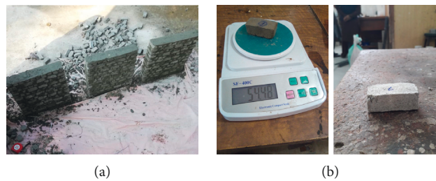
FIGURE 2: Brick masonry unit and wallettes used for basic testing of masonry constituents. (a) Masonry wallettes. (b) Brick unit.
