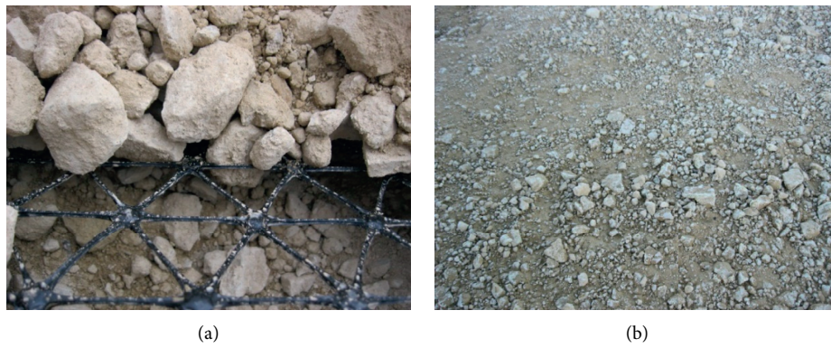
FIGURE 6: (a) C-stone and geogrid and (b) C-stone unstabilized test sections.
