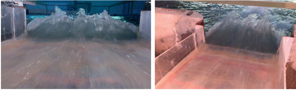
FIGURE 3: Interaction effect of jet flow with shockwaves in flip bucket area.
