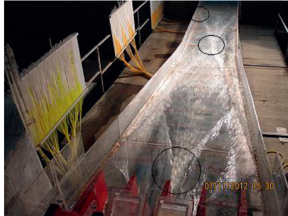
FIGURE 7: Flow and location of triple waves for two open middle gate modes.
