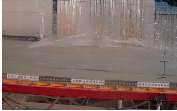
FIGURE 19: Separation of wave 2 from the main core of water flow.
