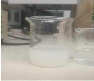
FIGURE 2: TBP/OK and H 3 PO 4 emulsion.
