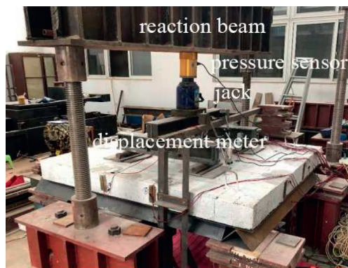
FIGURE 4: Field diagram of test loading.
