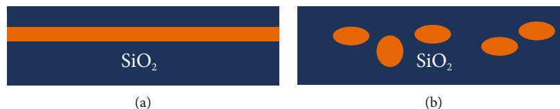
FIGURE 9: Schematic view of two potential interpretations of complex composition in PECVD Si layer: (a) continuous crystalline silicon “sublayer” and (b) matrix of silicon nanocrystals, both within the oxidized PECVD Si layer.
