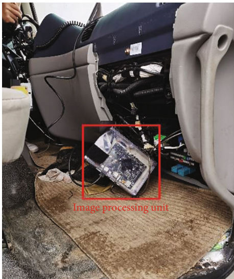
FIGURE 10: Deployment of image processing unit in experiment.
