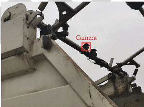
FIGURE 11: Deployment of camera in the experiment.
