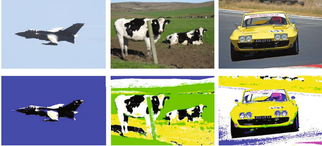
FIGURE 1: CN label sketch map. The first row is the original images, and the second row is the corresponding labeled images by CN.
