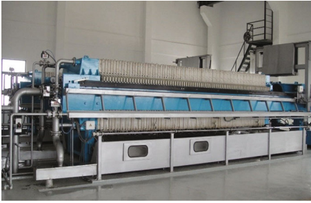
FIGURE 2: Diaphragm filter press.
