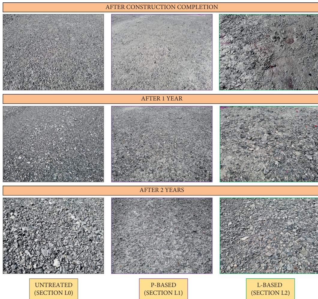
FIGURE 11: Surface appearance of the tested road sections during a two-year time span (the maximum size of the rock aggregates is 32 mm).
