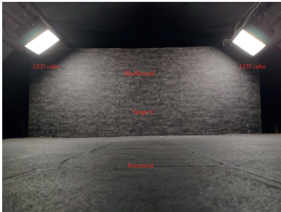
FIGURE 10: Schematic diagram of the simulated tunnel.
