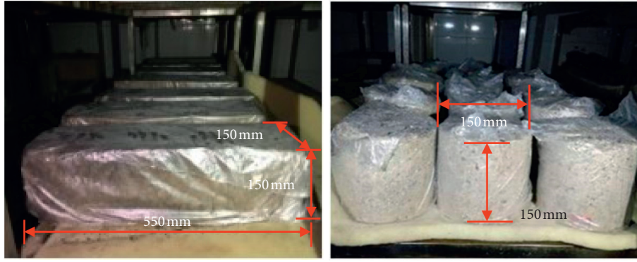
FIGURE 2: Preparation of cement-treated aggregate specimens.
