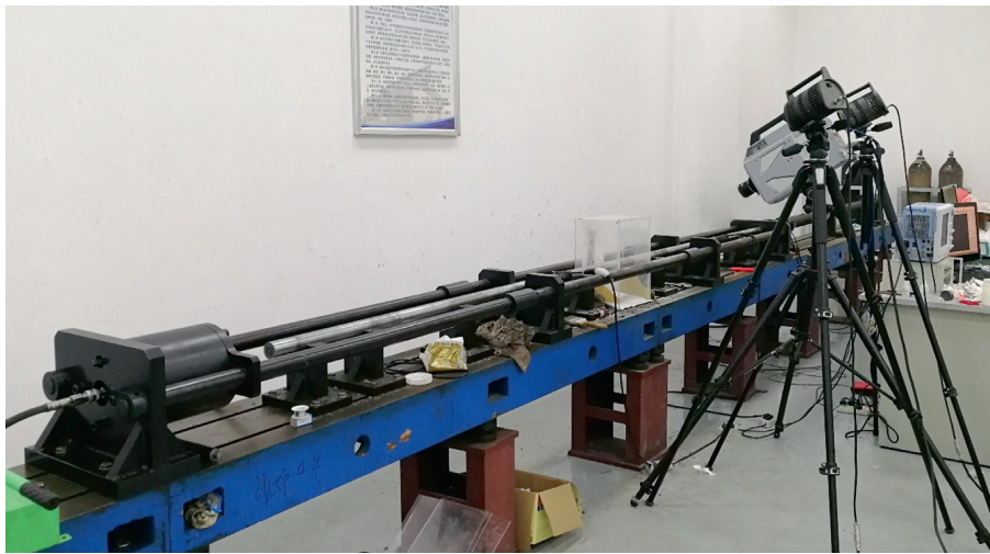
FIGURE 2: SHPB test system.
