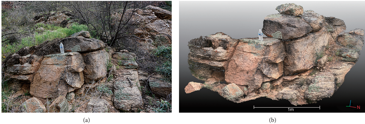
FIGURE 8: Point clouds of rock block sample generation by photogrammetry. (a) Rock block samples that were taken at the bottom of the Thimble peak. (b) Point cloud data of the rock block samples generated in Pix4D and segmented in CloudCompare software.
