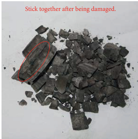
FIGURE 10: Modified epoxy resin filling.
