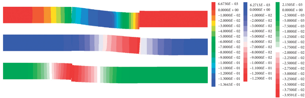
FIGURE 12: Subsidence trend chart of key block broken after roadway excavation based on three groups of models (from top to bottom, model ①, model ②, model ③).
