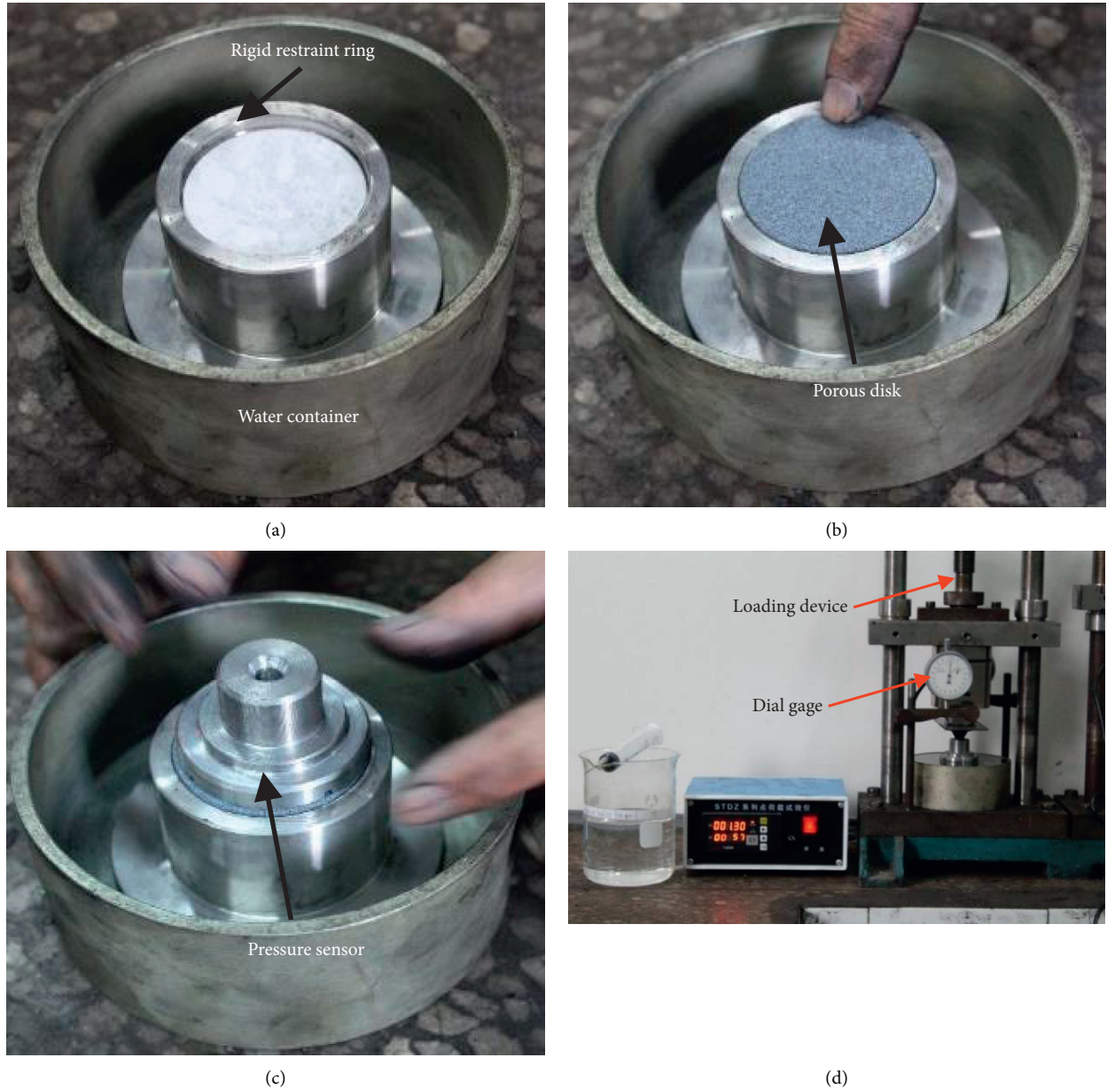
FIGURE 2: Swelling test apparatus.
