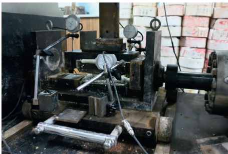
FIGURE 6: Displacement sensor installation photo.
