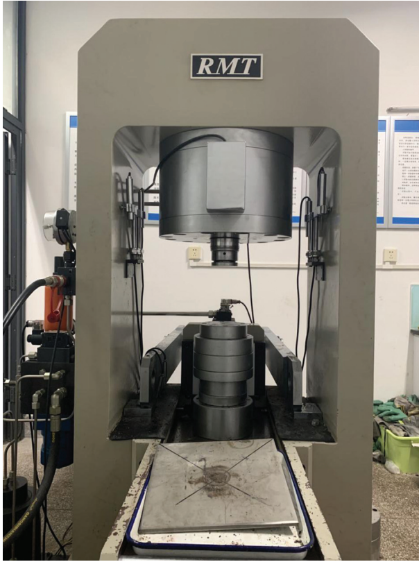
FIGURE 1: The RMT-150C rock mechanics test system.
