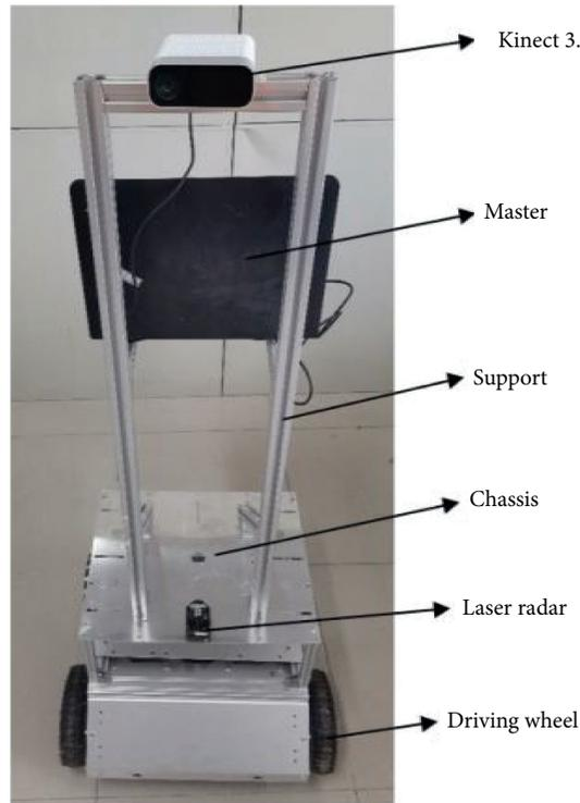
FIGURE 6: Experimental platform of robots.
