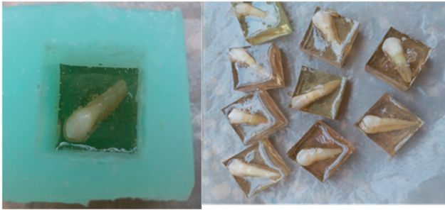
FIGURE 1: Mounting the specimens.
