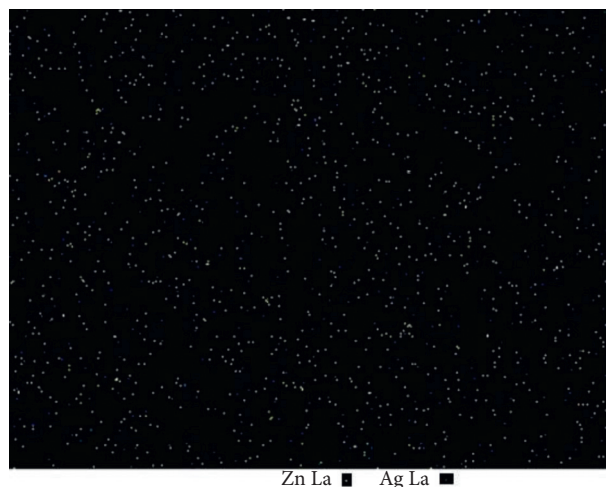
FIGURE 2: Zn and Ag map of the resin composite containing 10 wt % Ag/ZnO. Light yellow spots represent Zn, and blue ones represent Ag element.
