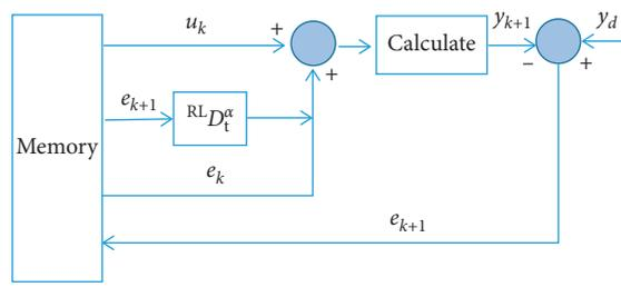
FIGURE 1: Block diagram of the open- and closed-loop  $PD^\alpha$ -type ILC algorithm.
