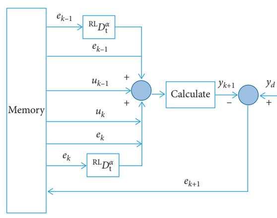
FIGURE 2: Block diagram of the second-order  $PD^\alpha$ -type ILC algorithm.
