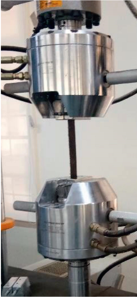
FIGURE 1: Tensile test of the BFRP specimen with a universal testing machine.
