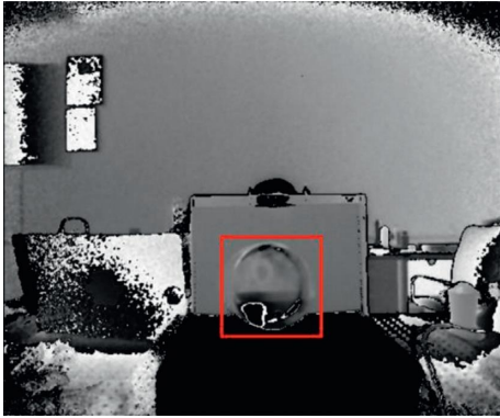
FIGURE 5: Examples of holes in the depth map. The object in the red box is transparent materials.
