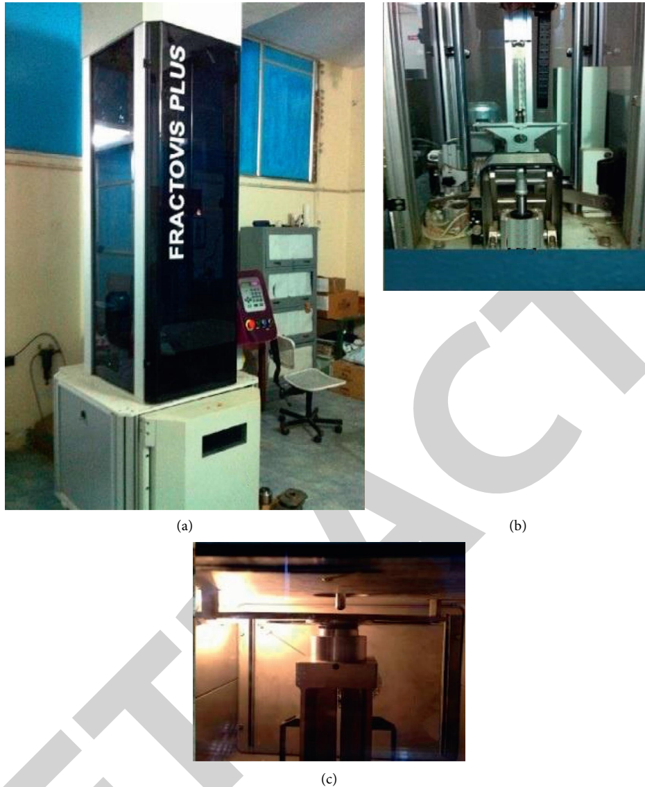
FIGURE 1: (a) Fractovis instrumented impact tester. (b) Impact striker with the load cell. (c) Specimen holder, clamped during impact.
