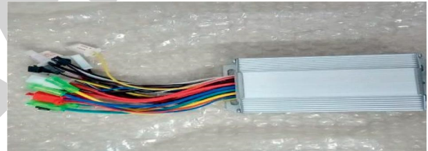
FIGURE 7: Typical model of the motor controller.
