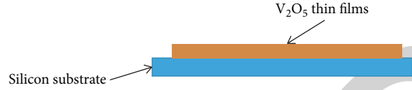
FIGURE 1: V_2O_5 thin film deposition using PLD.
