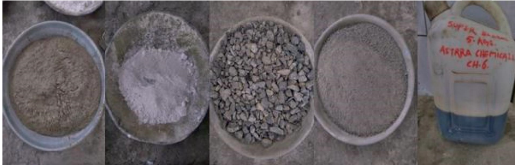
FIGURE 1: Concrete constituents (cement, sand, silica fume, fly ash, aggregate, and superplasticizer).
