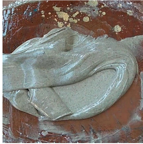
FIGURE 7: Mixture of epoxy resin, quartz powder, and rice husk ash.
