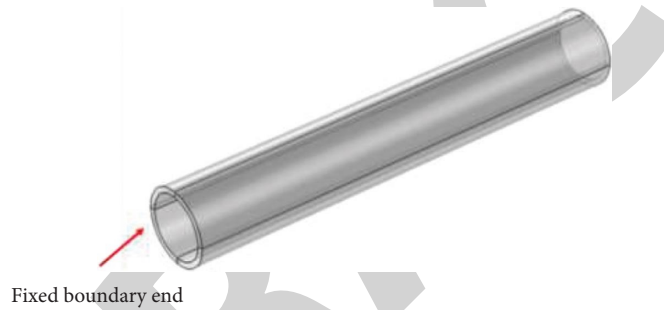
FIGURE 6: Fixed-free boundary fundamental frequency analysis (one end is fixed and another one end is free).
