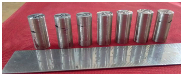
FIGURE 4: Pin-on-disc samples extracted from laser hardfaced deposit.
