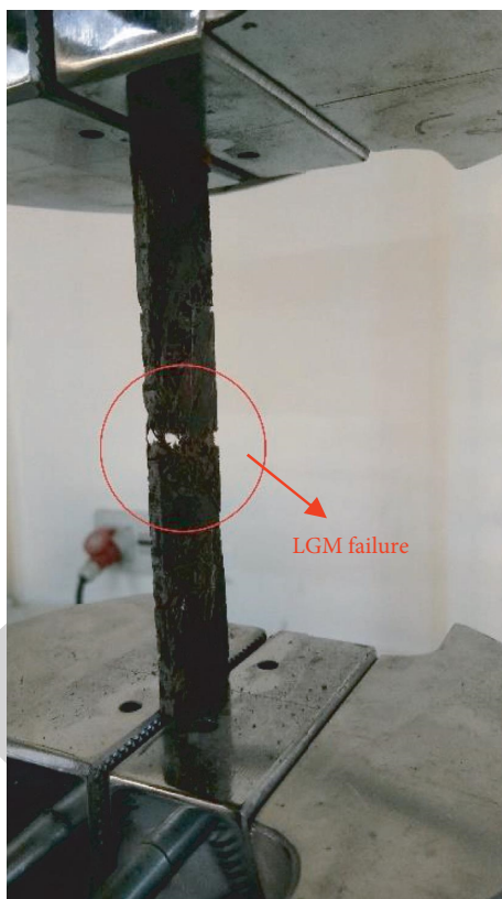
FIGURE 8: Failure of the BFRP specimen under tensile loading.
