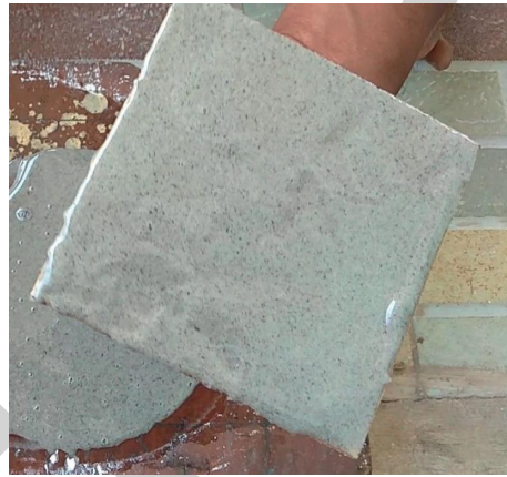
FIGURE 8: Material coated using the epoxy mixture.
