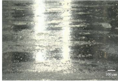
FIGURE 26: The whole morphology of the hole.
