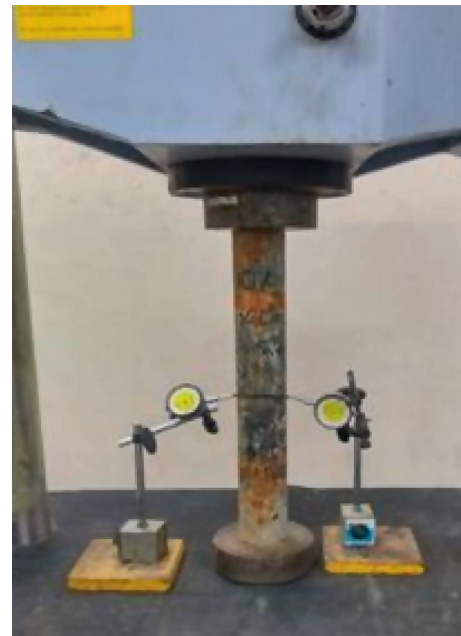
FIGURE 3: Test setup for the composite column.
