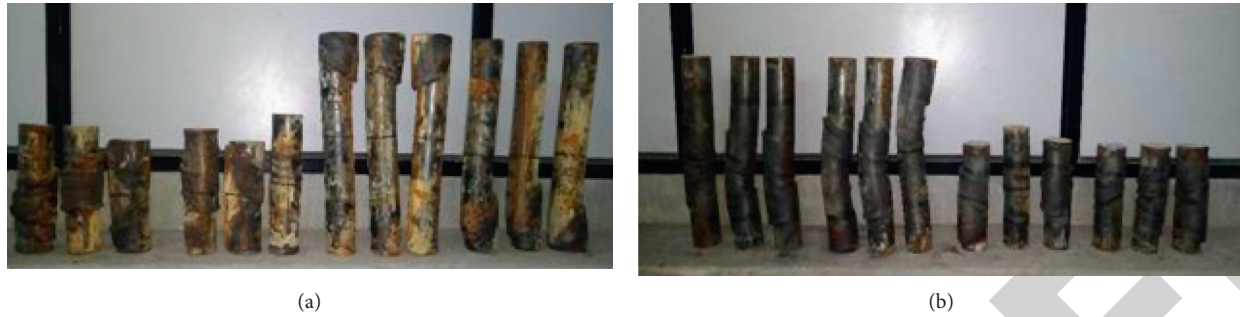
FIGURE 12: Mode of failure for composite columns of 1.5 mm and 2 mm steel tube thickness.
