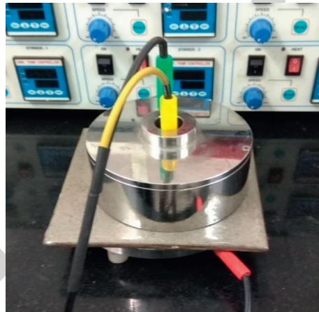
FIGURE 10: Testing of the press board coated with epoxy coating.
