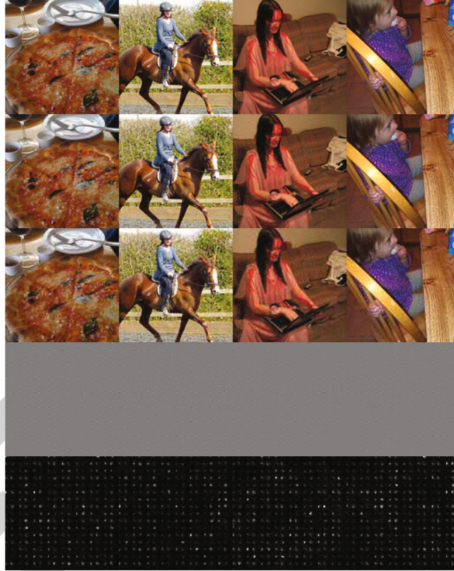
FIGURE 3: Examples of showing the robustness of the model against JPEG compression ( Q = 50 ) with experimental results. From top to bottom are the cover images, the encoded images, the noised images, the residual between cover images and encoded image, and the normalization of the residual signal.
