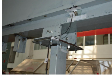
FIGURE 2: Connection of fixed bearing pier.
