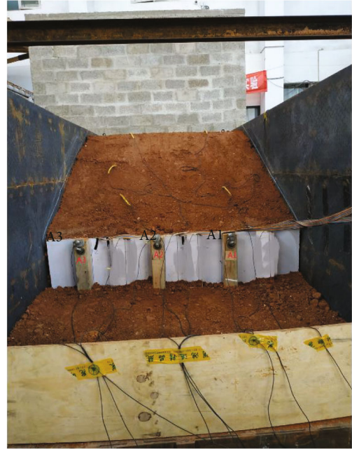
FIGURE 3: Assembly of the acceleration sensors.
