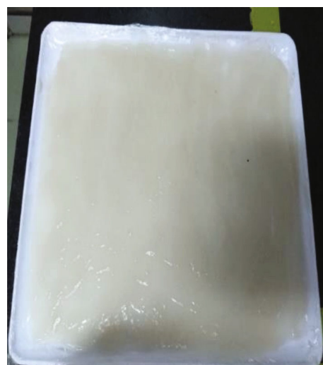
FIGURE 2: Flattened viscous bioplastic on the PE film coated tray.
