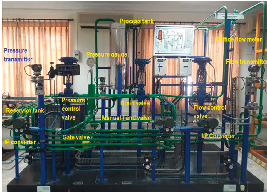
FIGURE 1: Experimental hardware for water distribution system.
