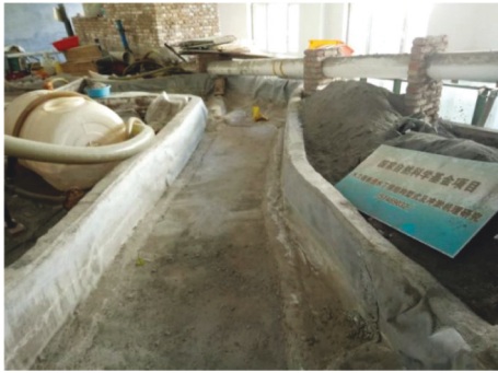
FIGURE 1: Front view of the flume model.
