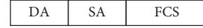
FIGURE 2: ACK frame at the data link layer is used for reliable communication.
