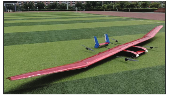
FIGURE 14: Physical prototype of grazing UAV.
