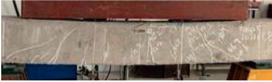
FIGURE 11: Failure pattern of the control beam.
