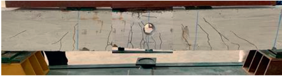
FIGURE 12: Failure pattern of beam BCOF.
