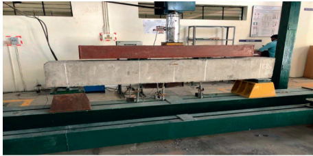
FIGURE 4: Test setup of the control beam.
