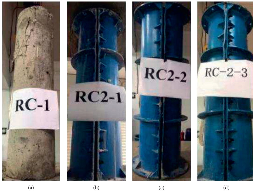
FIGURE 6: Failure modes of typical specimens.
