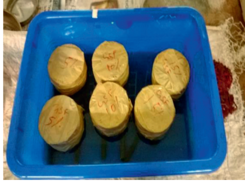
FIGURE 6: Specimens for the sorptivity test.
