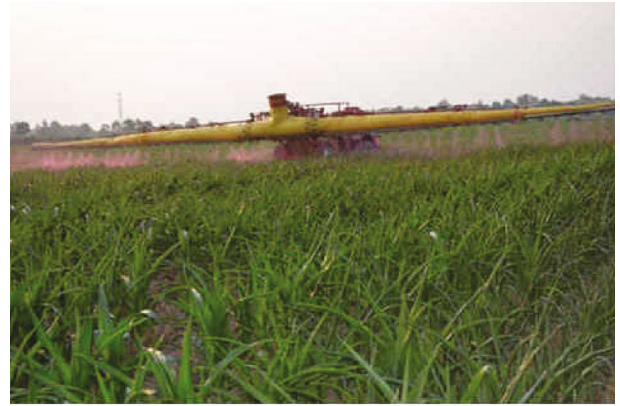
FIGURE 9: Experiment without auxiliary airflow.
