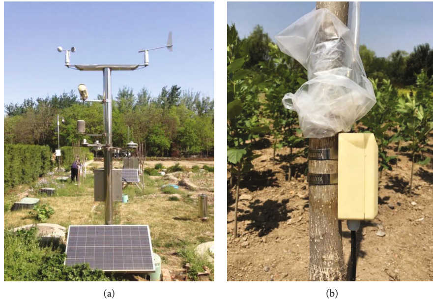
FIGURE 1: (a) The installation of environmental sensors. (b) The installation of SWR sensor.
