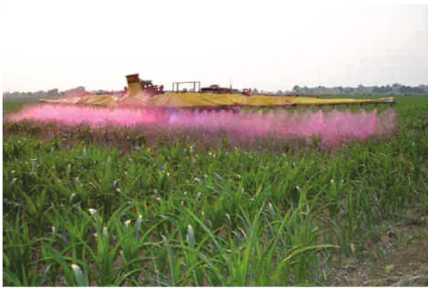
FIGURE 8: Experiment with auxiliary airflow.
