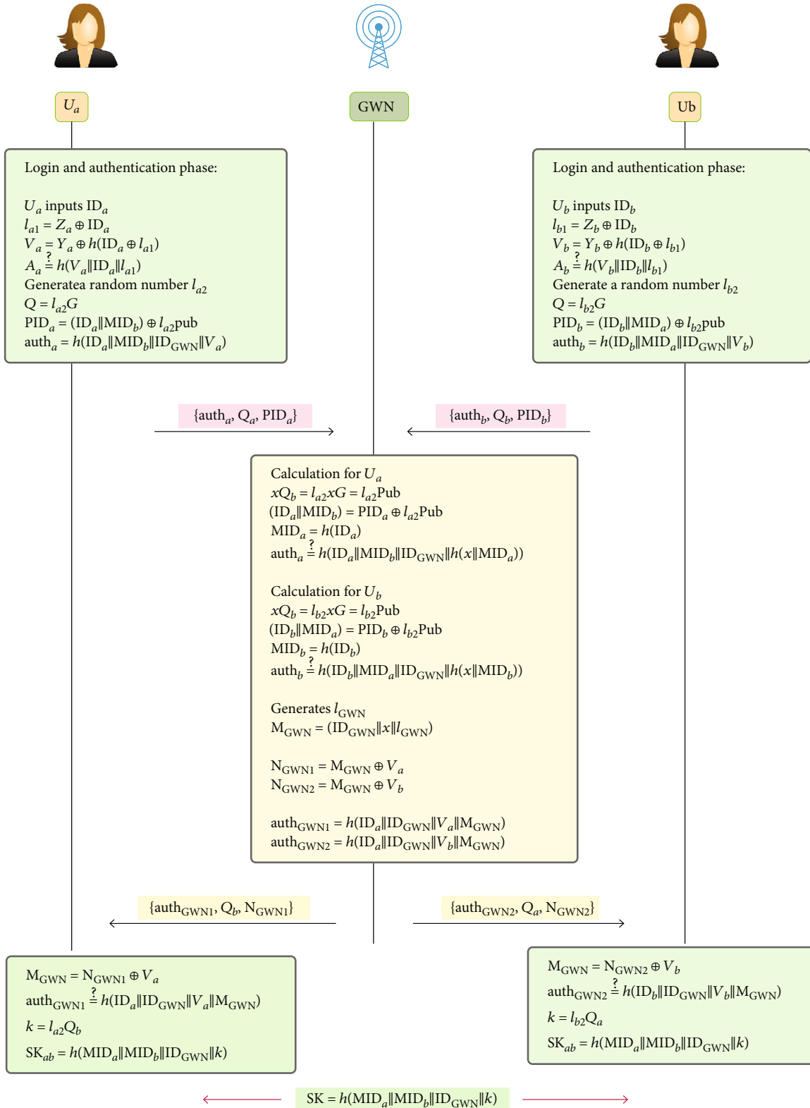
FIGURE 3: Login and authentication process of U_i .
