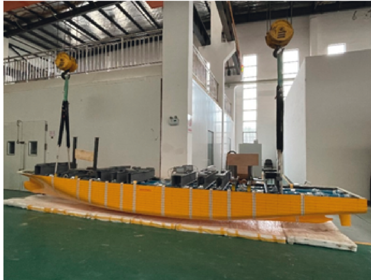
FIGURE 8: Different suspending patterns in the measurement of the modal shapes.
