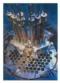
FIGURE 4: WWER-1000 mockup general view on reactor LR-0.
