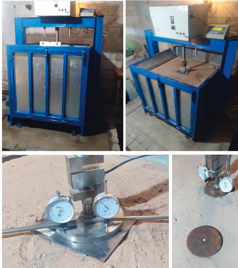
FIGURE 4: Pi simulator for large-scale and load plate tests with displacement and dynamometer sensors.
