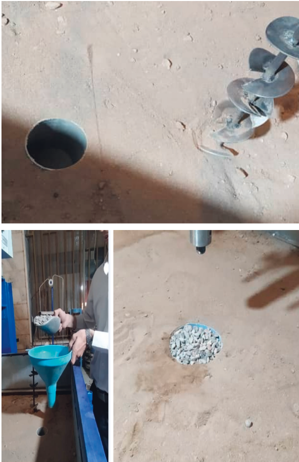
FIGURE 5: Steps of making a stone column in the laboratory.
