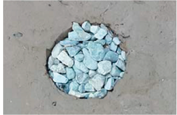
FIGURE 1: Sample of a stone column made in laboratory conditions [1].
