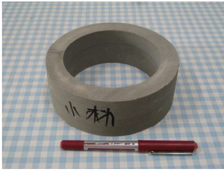
FIGURE 6: Hollow cylinder sample of the Tangenshan sandstone.
