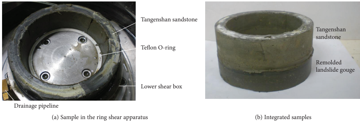
FIGURE 8: Sample arrangement for the ring shear test.
