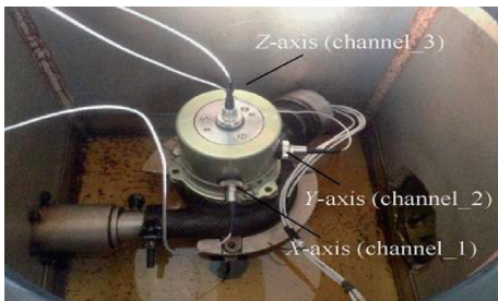
FIGURE 9: The installation of the airborne fuel pump in the testbed.
