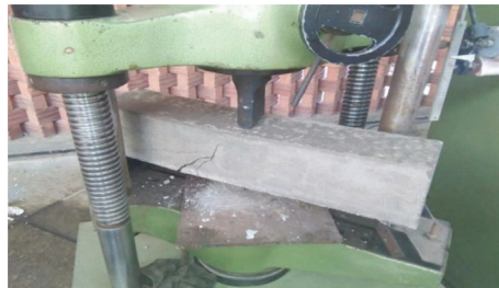
FIGURE 12: Performing flexural test (source: author).
