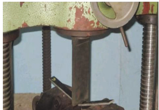
FIGURE 4: Flexural testing of the specimen sample.
