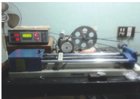
FIGURE 3: Tensile test-digital tensometer setup.
