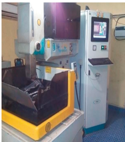
FIGURE 2: Wire-cut EDM machine ULTRACUT S2.
