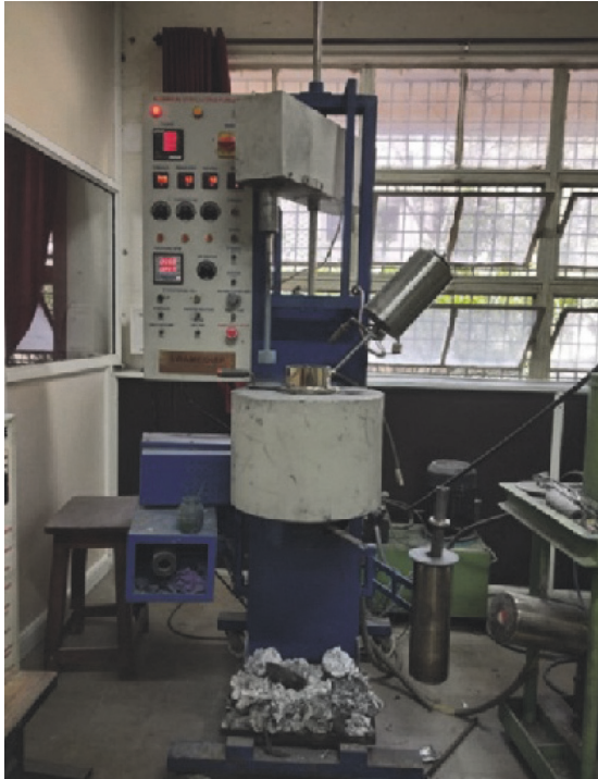
FIGURE 2: Experimental setup of the stir casting process.
