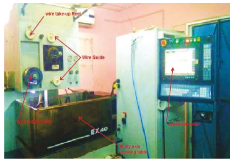
FIGURE 4: Wire cut EDM machine setup.
