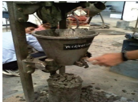
FIGURE 8: Vee-Bee test setup (source: author).
