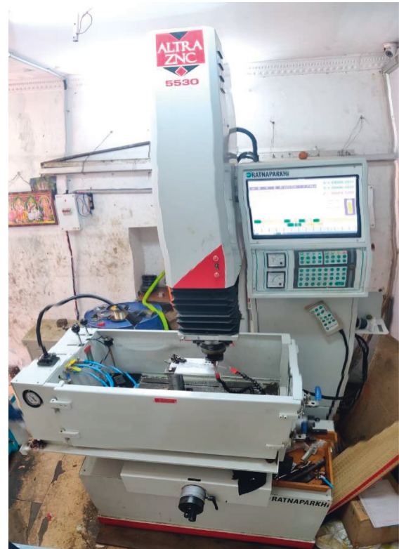
FIGURE 1: Electrical discharge machine used for this investigation.
