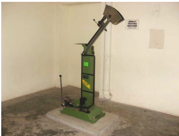
FIGURE 6: Impact testing of the sample specimen.
