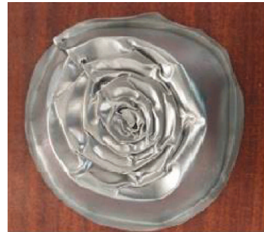
FIGURE 2: Crushed patterns of cones.
